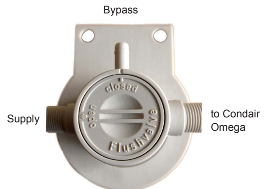
Fig. 21: Set valve to "Supply" (operating position)
