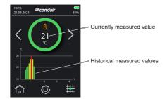
Display of the 4-hour history of the values - here, for example, the temperature readings.
