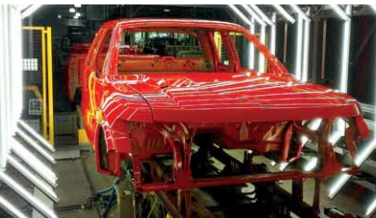
Ford's Automated Inspection System, which debuted at Dearborn Truck Plant, uses up to 16 high-resolution cameras, plus fluorescent lamps
