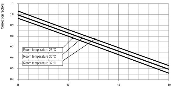
Difference between water inlet temperature and room temperature (°C)
