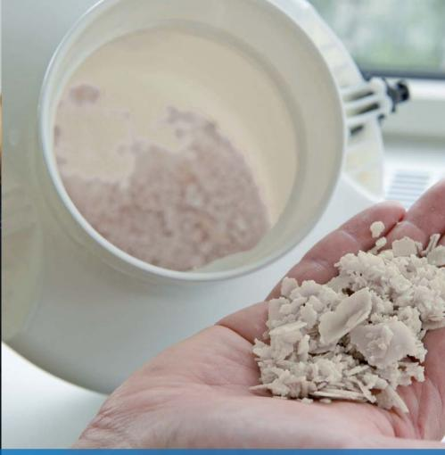
Collected scale is easily removed from the system in minutes
