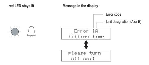
Note: If the unit is in the display or setting level the error message in the display will be suppressed.
