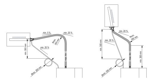
Initially, lead the steam hose at least 300 mm perpendicularly upward above the top edge of the humidifier, then lead the hose with a minimum upslope of 20% and/or a minimum downslope of 5% to the steam distribution pipe.
