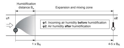
The calculation of the humidification distance " $B_N$ " is dependent on several factors. For a rough estimation of the humidification distance " $B_N$ ", the following table is useful. Recommended standard values listed in this table are based on a supply-air temperature range of 15 °C to 30 °C. The values given in bold type only apply to steam distribution pipes 81-..., the values in brackets apply to the OptiSorp steam distribution system.
