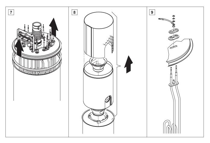
7. Carefully lift off the cover with the heating rods.
