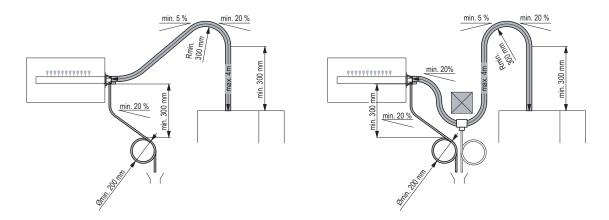
Initially, lead the steam hose at least 300 mm perpendicularly upward above the top edge of the humidifier, then down to the steam distribution pipe with a minimum slope of 5 %.
