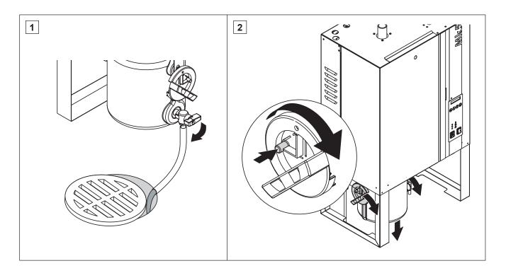
1. Empty the lime collector tank via the drain valve.
